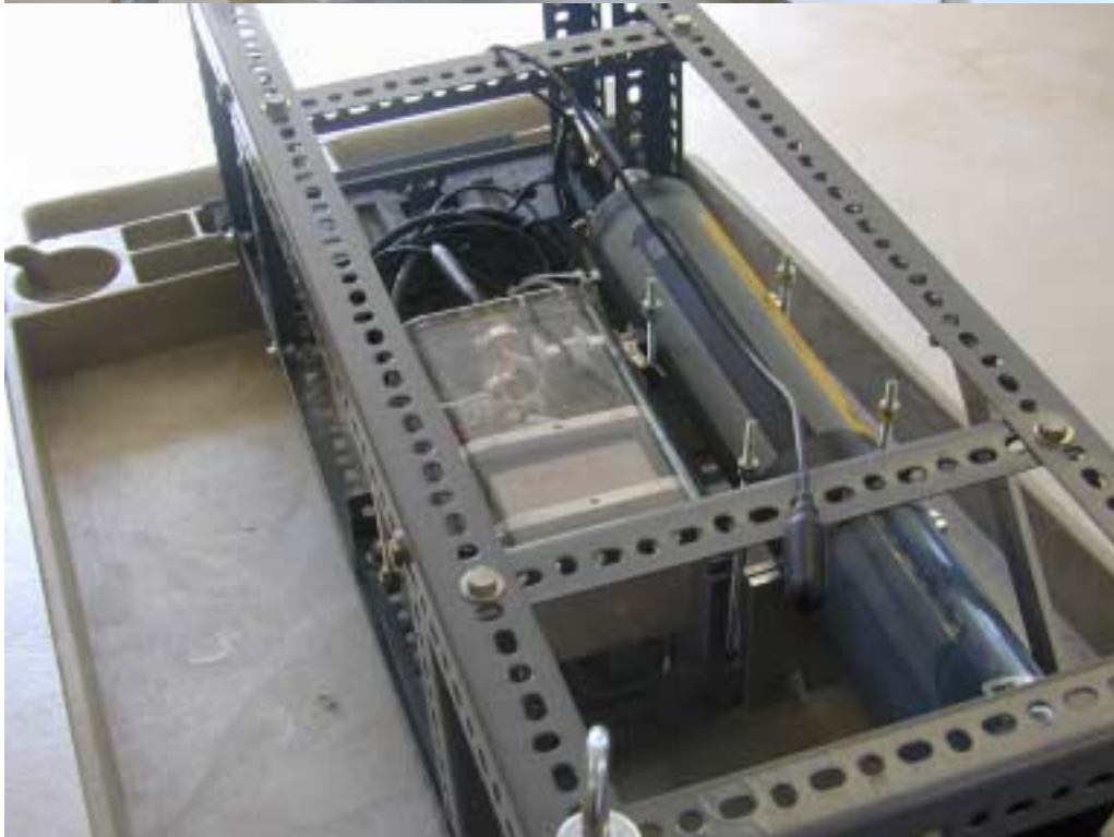
Figure 4 (top and bottom). Top – the deployment frame with YSI data sonde and FABULS housing. Bottom – an end view of the frame, showing location of the FABULS and sonde, with HTI hydrophone at top. Prior to deployment, angle iron clamps and cable ties are used to secure the housing, sonde, and hydrophone to the frame. The frame is weighted and a marker float is attached prior to deployment.
