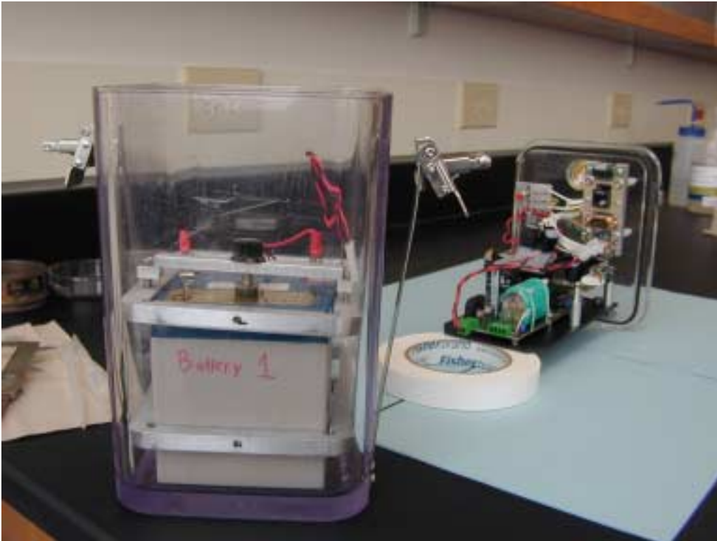
Figure 2. Photos of the FABULS in laboratory, pre-deployment. The Ikelite housing (foreground) contains a rechargeable sealed lead acid 5 amp-h battery with supports to hold the battery in place. The Viper computer and UPS are mounted to the housing's lid (background), with internal connections for power, serial and Ethernet cables. To set-up and program the Viper, the power cable is connected to the battery leads and a laptop computer is connected to the internal serial port. A red reset button is present for resetting the computer during pre-deployment procedures.
